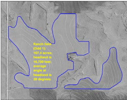
A Kastens field that is much less efficient than squares, triangles, or circles a single 90° pass with a sprayer gets 20% of the field!
